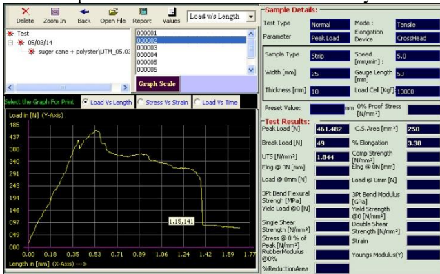
Composite Material: 30% CFF & 70% Phenylester.
